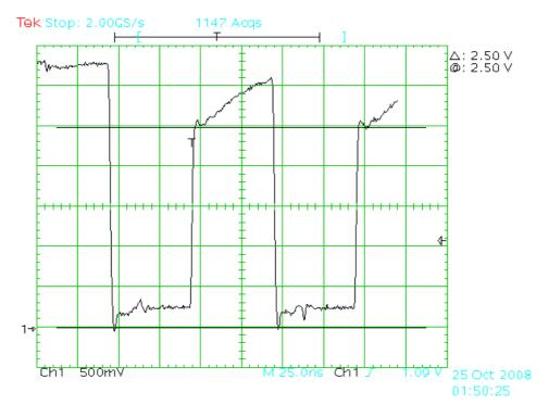
This is a scope capture of the ADC clock which is driven at 10MHz, the cursors are at 0V and 2.5V.
