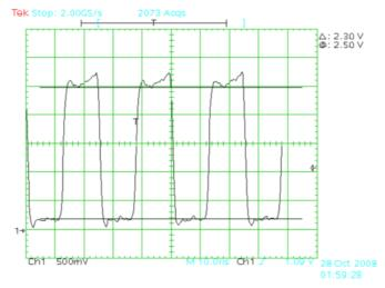
3) SPI DOut toggled at 80MHz. Cursors at 0V and 3.2V. This was taken with no load on the output.
