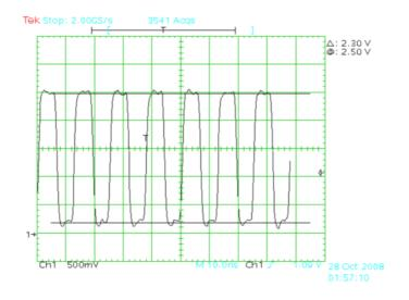
2) GPIO Pin toggled at 40MHz. Again the cursors are at 200mV and 2.5V.
