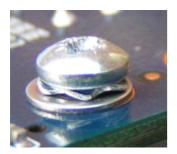
To support the other end of the GPIB please install the 17mm standoffs provided with the other two M6 screws provided. The length of these is chosen to match the standoffs provided with the CIII starter board so these must be fitted too.
