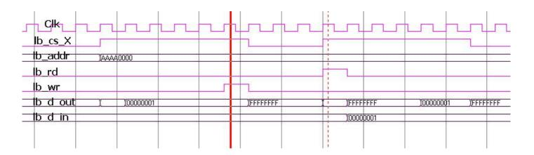
The write occurs on the cycle indicated by the first solid cursor, the read on the dotted second. The write cycle is writing 0x00000001 to a local address. **The lb\_d\_in from a read is registered in at the end of the clock cycle following the active lb\_rd signal.** It can be seen that the value written during the write cycle is returned. It is recommended this be registered synchronously against the address, chip select and read signals.
